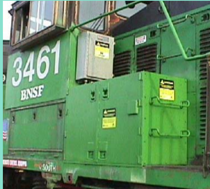
Diesel-Driven Heating System
